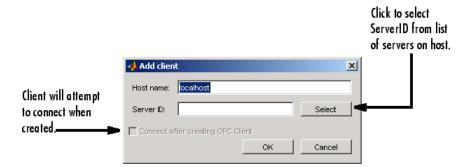
When you supply a hostname, you will be able to select the Server ID from a list, by clicking **Select**. Using the Add client dialog, you can also automatically attempt to connect to the server when the client is created, by checking **Connect after creating OPC Client** before clicking **OK**.
