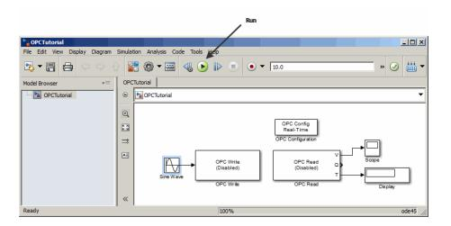
The model writes a sine wave to the OPC server, reads back from the server, and displays the wave in the scope trace. In addition, the quality value is set to 192, which indicates a good quality (see Appendix A, "OPC Quality Strings").
