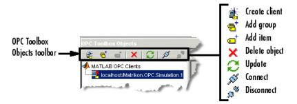
Click **Connect** in the **OPC Toolbox Objects** toolbar. If the client is able to connect to the server, the icon for that client in the **OPC Toolbox Objects** tree will change to show that the client is connected. If the client could not connect to the server, an error dialog will show any error message returned.
