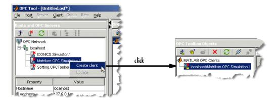
The name of the client (displayed in the **OPC Toolbox Objects** pane) is <code>Host/ServerID</code>, where <code>Host</code> is the hostname and <code>ServerID</code> is the Server ID associated with that client. In this example, the client's name is <code>'localhost/Matrikon.OPC.Simulation.1'</code>
