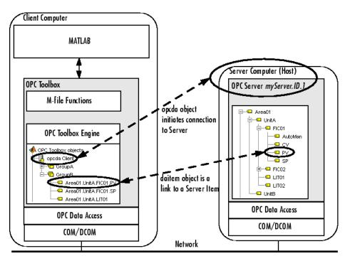
The opcda client object establishes the connection between OPC Toolbox software and the OPC server, using OPC Data Access Specification standards. The standards are based on Microsoft COM/DCOM interoperability standards.
