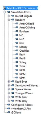
An item is usually represented by its fully qualified item ID (FQID) within the name space. An FQID is usually comprised of each level of the item's hierarchy separated by periods. For example:
