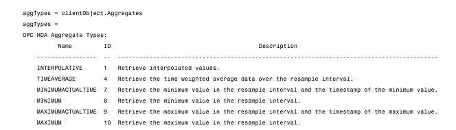
In the previous example, the server supports six types of aggregate.
